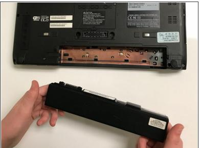
• After, you unlock both sides of the battery, gently slide the battery off by pulling towards yourself.
