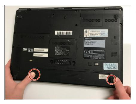
Unlock the battery by sliding both tabs at the same time.
