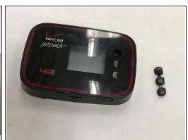
Now that the motherboard is out, the buttons should come easily out of what's left of the device. If they do not fall out once the motherboard is out, simply poke the buttons from the front and they should separate from the device.
