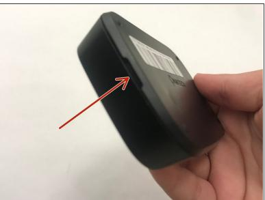
Hold the device with your non-dominant hand, looking at the back of the device, taking note of the small notch along the edge.
