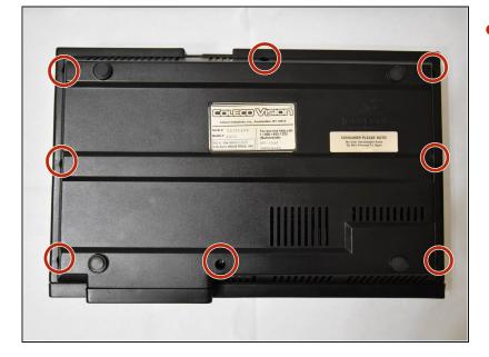
Flip the console upside down and remove the eight 15mm Phillips #1 screws.
