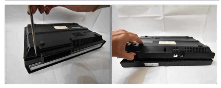
• Use the metal spudger along the bottom rim of the front panel to safely remove the top of the console. Set aside the top.
