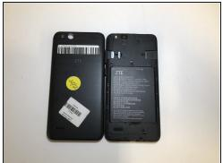
Using the opening tool, pry open the rear cover from the crease at the bottom left corner.
