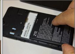
Remove the battery with an opening tool or fingernail.
