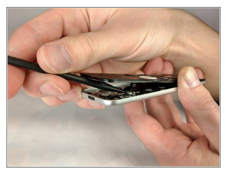
• Unlatch the connector that binds the touch screen and logic board.
