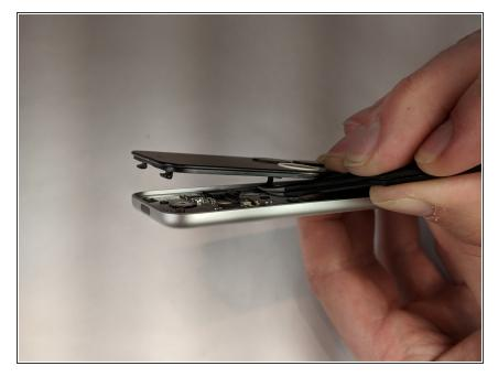
• Use tweezers to pull off the connector that binds the touch screen to the logic board.
