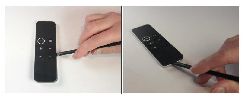
Using a spudger, gently lift the face of the remote. Starting from the bottom and working your way to the top.
