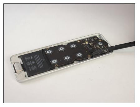
Using a plastic spudger, gently remove the logic board from the case of the remote.
