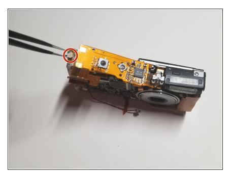
• Lift up the button that connects to the power button of the camera so you can remove the control panel.
