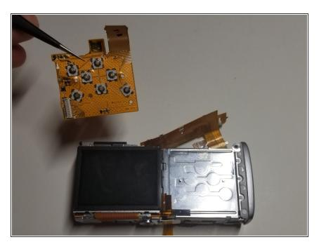
• Remove the control panel from the camera.
