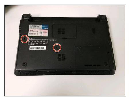
Use the Phillips #0 screwdriver to remove the two screws on the back of the laptop.
