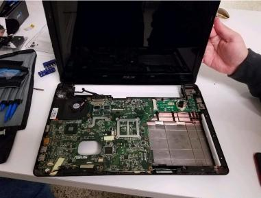
• Use the spudger to pry up the front panel from the back panel.
