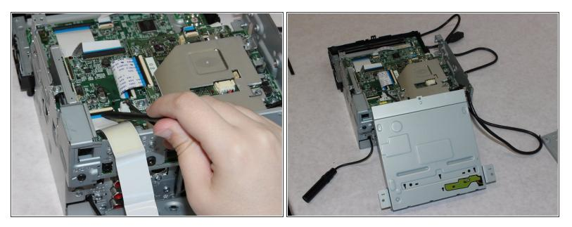
Flip up the black clasp with a spudger to disconnect the large white ribbon cable connecting the CD drive to the board underneath.
