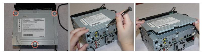
• Unscrew the three 5mm screws from the top of the device using a Phillips #1 screwdriver.
