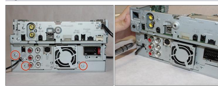
Unscrew the three 5.5mm long screws with a Phillips #1 screwdriver.
