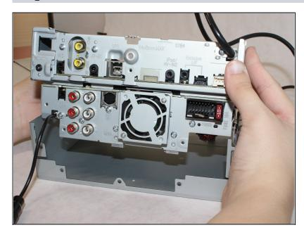
• Lift the top part of the unit up from the lower chassis.
