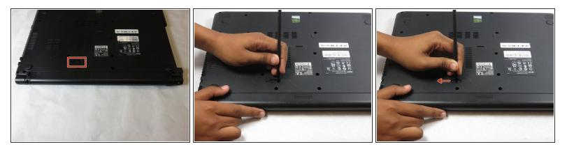
Use your finger or a spuger to pull the battery release switch.
