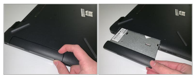
• Pull outwards on the disk reader to remove from main frame.
