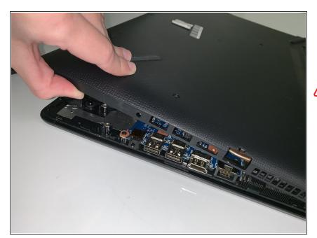
Lift back panel to access internal components.
