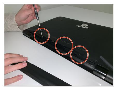
Use the Philips 0 screwdriver to unscrew the screws (7.51mm) that were underneath the battery.
