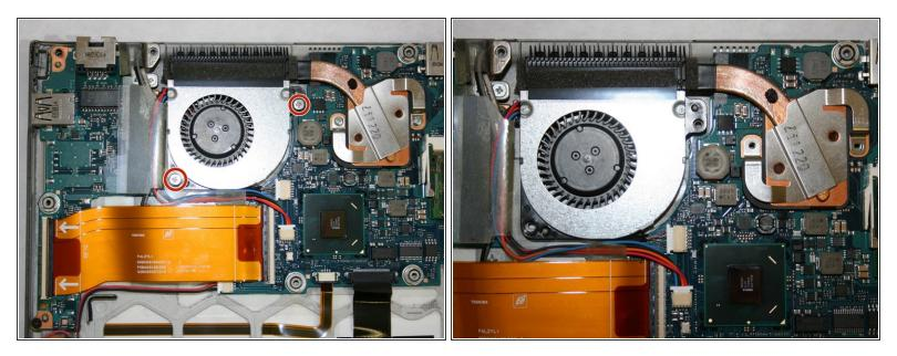
• Use a Phillips #0 screwdriver to remove the two 5 mm screws securing the fan.
