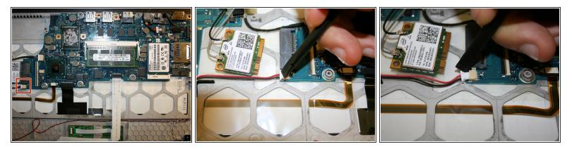
• Remove the CMOS battery connector cable (red/black) from its port using a Nylon Spudger Tool.
