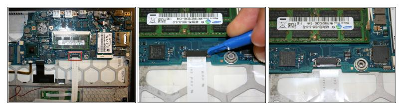
Disconnect the white cable from the port by using a Plastic Opening Tool.
