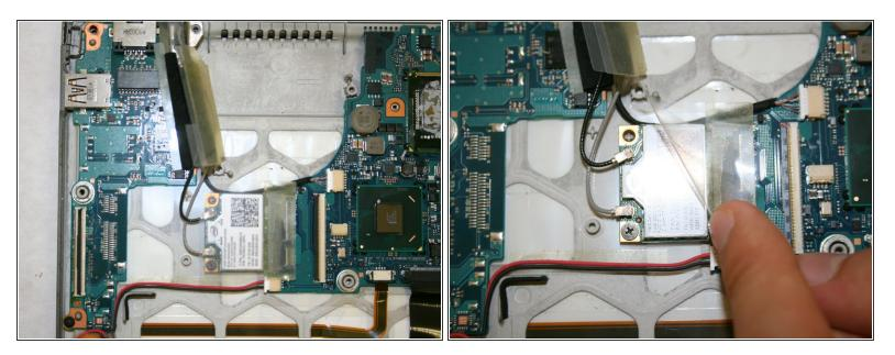
• Remove the clear tape covering the Wi-Fi card.
