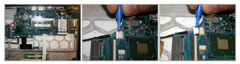
Disconnect the plug from the motherboard using a Plastic Opening Tool.
