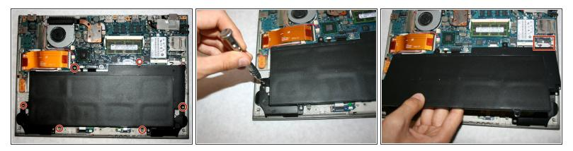
(i) The battery is the black rectangular piece in the bottom half of the device.
