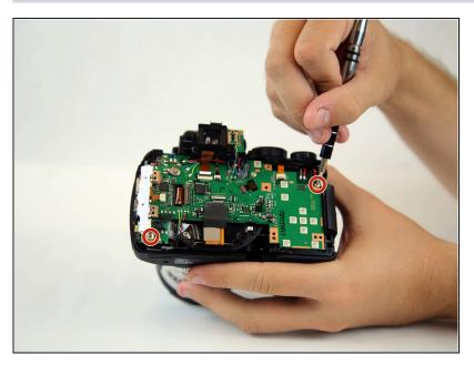
• With the Phillips #00 screwdriver, remove all screws.
