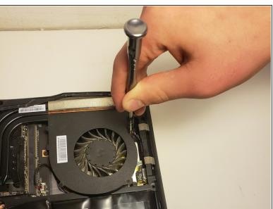
Remove the three 2.0mm screws using the JIS #0 screwdriver.
