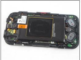
Once the back cover is removed, the (6) buttons along the side are going to fall out of place.
