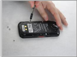
Remove the eight screws with a JIS #0 screwdriver.
