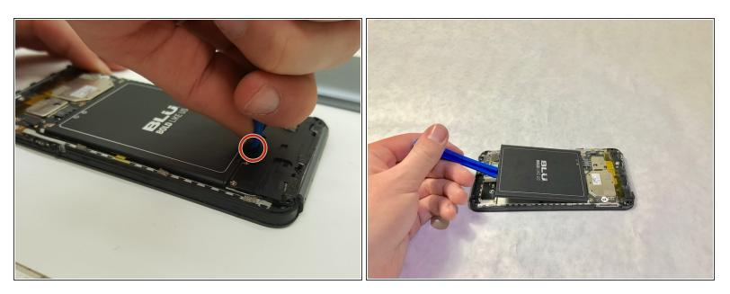
(i) There is a patch of adhesive underneath the battery, which can make it difficult to remove.
