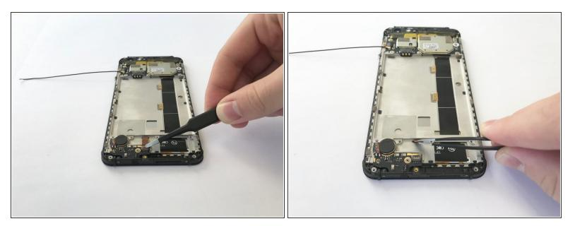
• Use a pair of tweezers to remove the orange data cable as shown.
