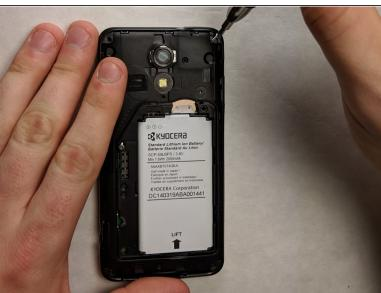
Remove six Phillips screws (screw length of 5.35 mm and screw head diameter of 2.95mm) on the back of the device using a Phillips #000 screwdriver.
