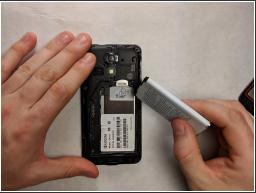
Remove the battery by popping it out of the phone by using your hands or the spudger to pry it up out of the case.
