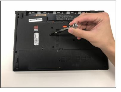
Using a Phillips #0 screwdriver, remove the 5.3 mm screw from the back panel.
