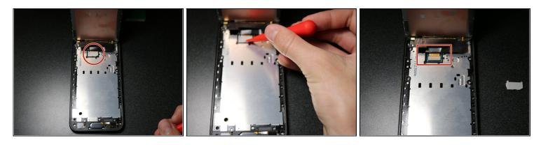
• Use your prying tool to slowly pry up on the **bottom right corner** of the white cable guard, exposing a thin ribbon cable connector.
