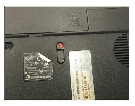
Switch the battery lock to show a <u>red</u> background with an unlock symbol
