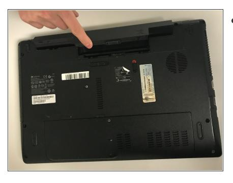
Remove the battery by lifting the battery out.
