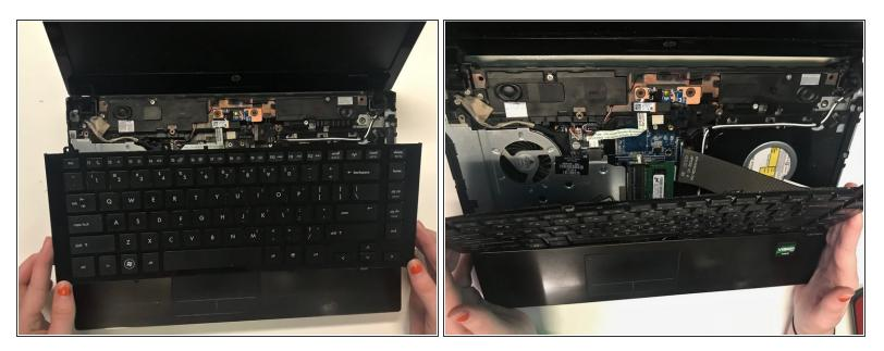
Carefully remove the keyboard by sliding it up towards the screen of the computer in order to release the keyboard ribbon cable.
