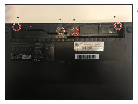
Remove the four 3 mm Phillips head screws that secure the switch cover in place.
