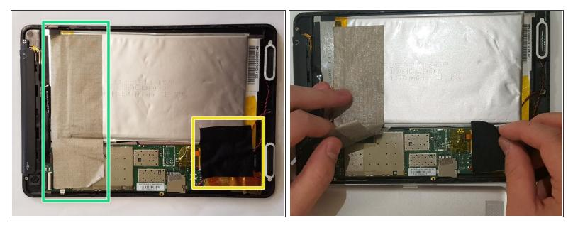
↑ The black tape is stuck to delicate wires; remove with caution.
