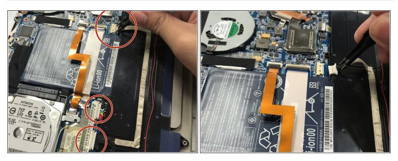
Unplug the three white plugs from their sockets using tweezers by pinching the plugs and pulling them outwards.
