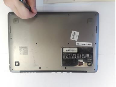
Remove the twelve 5mm screws with a Phillips #1 screwdriver.
