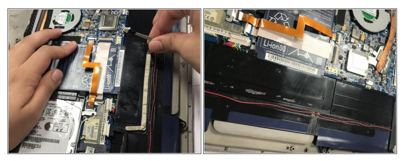
Pull upwards on the plugs located on top of your battery until they have completely come off.
