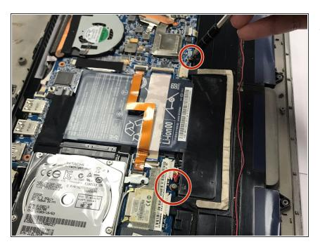
With the Phillips #1 screwdriver, remove the two 5mm screws located on either side of the battery.
