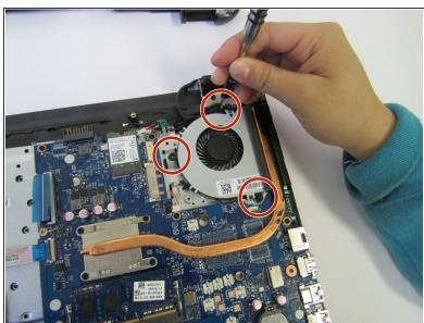
Remove the three Phillips head screws attached to the fan.
