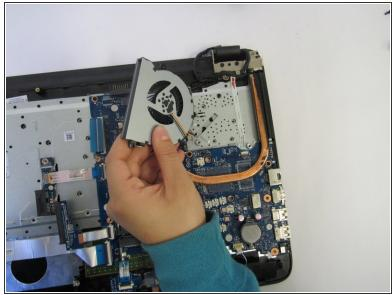
Remove old fan and replace with a new fan.
