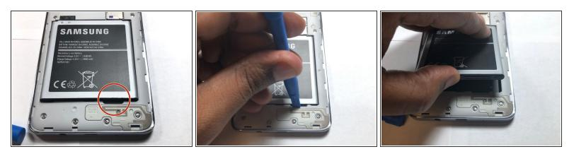
• Locate the battery notch and remove the battery, using either your finger or a plastic prying tool.
