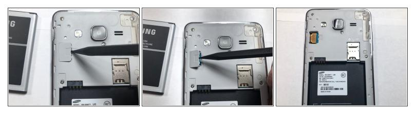
• Use the plastic Spudger tool to pry open the LCD ribbon cable cover.
