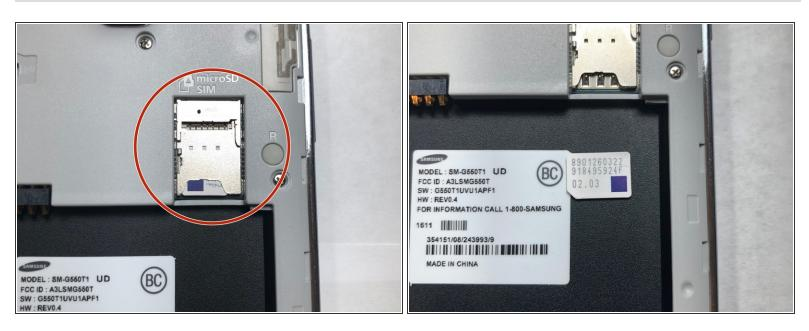
$\blacksquare$  Before disassembling the phone, take out the SIM card and microSD card.
