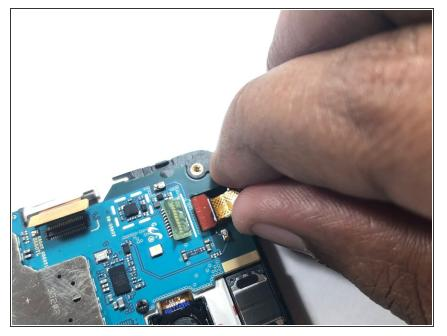
Once the camera is out of the housing, disconnect the camera from the logic board.
