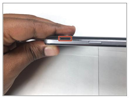
• Locate the side notch that allows you to open the back casing.
