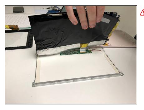
Mhile you're peeling the adhesive back, be careful because the display is connected by a cable on the right.
