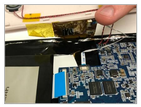
Peel back the touch interface chip (which is on the top right of the motherboard, covered in yellow tape.)
