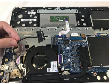
Use your fingers to lightly pull the cable and disconnect it from the motherboard.
