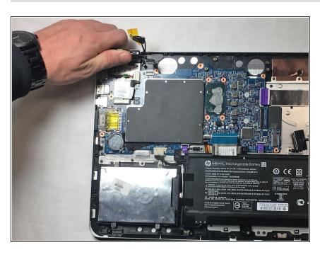
Using your hand, lift the screen hinge located in the top left corner.
