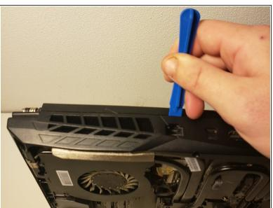
Insert the plastic opening tool into the side of the laptop above the fan, and lightly pry it up.
