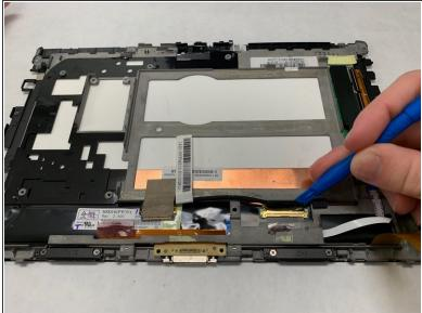
Use fingers, plastic opening tool, or metal spudger to lift the clip securing the display cable and remove by sliding it out.
