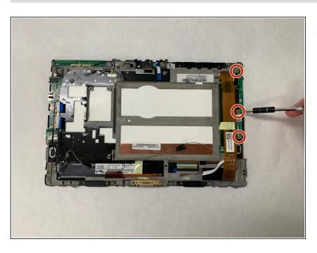
Use a Phillips #00 Screwdriver to remove the three 3 millimeter screws securing volume button board.
