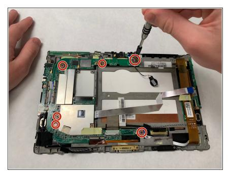
Use a Phillips #00 Screwdriver to remove the six 3 millimeter screws securing the motherboard to the screen.
