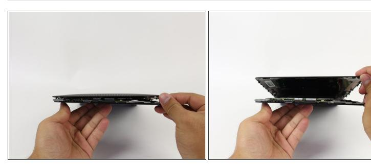
Remove back panel by pulling away from the remaining device.
