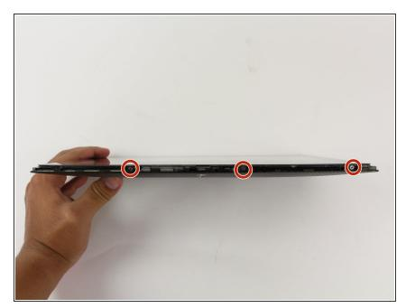
Use a Phillips #00 Screwdriver to remove the three 3 millimeter screws securing the front panel to the back panel found above the camera area, on the top portion of the tablet.
