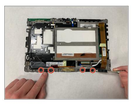
Use a Phillips #00 Screwdriver to remove the four 3 millimeter screws securing the two black ports at the bottom.
