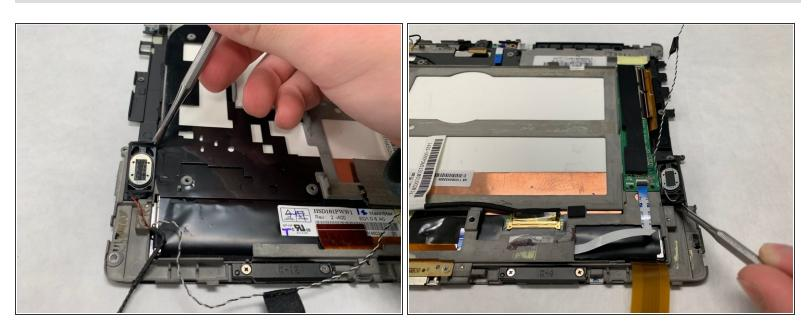
Use fingers, plastic opening tool, or metal spudger to lift the glued-in left and right speaker.
