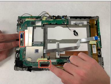
• Use fingers, plastic opening tool, or metal spudger to lift the clips to the ZIF connector. Remove the ribbon cables attached underneath.
