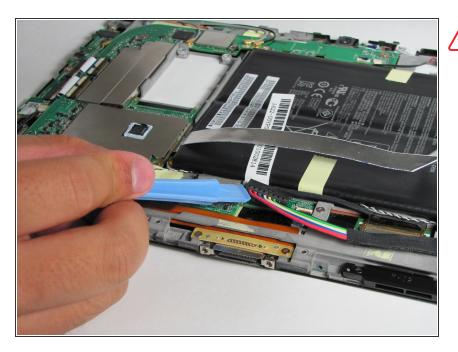
**Do NOT** pry the battery connector upward as shown in this photo. Instead, pull the connector straight out (in the direction of the wires).
