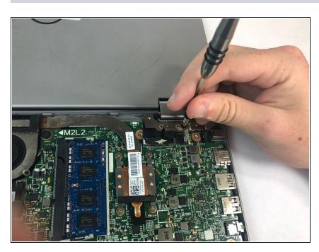
• Remove the 2 5.6mm PH0 screws.
