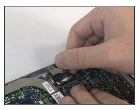
Use the pull tab to disconnect the display cable from the system board.
