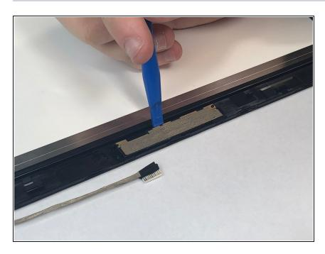
Use a plastic opening tool to take the camera module off the display.
