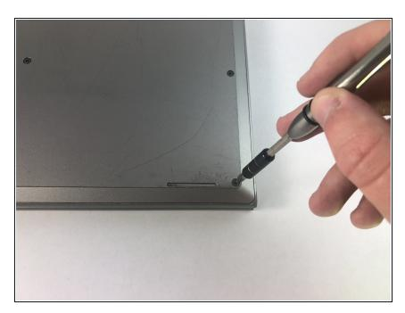
Remove the nine 7.6mm PH0 screws on the cover.
