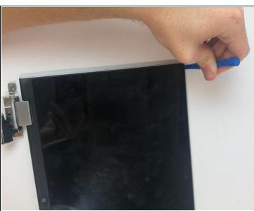
Use a plastic opening tool to take the display panel assembly off the display back cover and antenna assembly. Start from the top.
