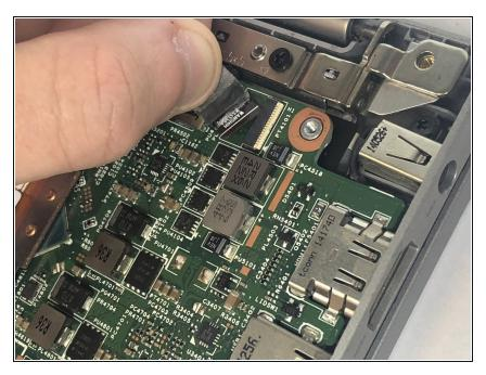
Pull the windows button board cable from the system board.
