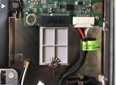
• Use a plastic opening tool to remove the card from the board. The card is now free to be taken out.
