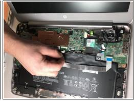
Disconnect the battery cable shown in the first picture before moving on. This can be done with an opening tool if necessary.
