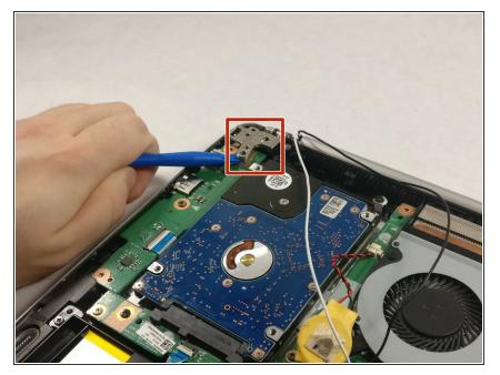
Using a plastic opening tool, pry open the hinge shown until your fingers can fit under it.
