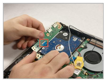
Disconnect the plate from the shown connector. The USB port plate is now disconnected from your device.
