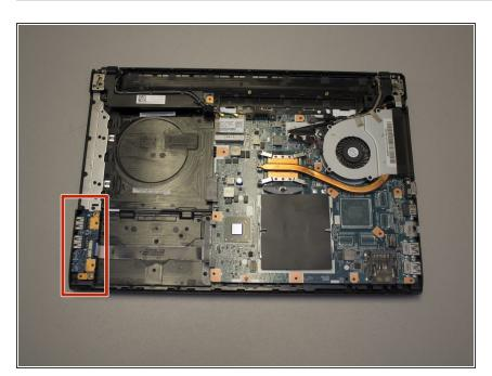
Locate the I/O card in the bottom left hand corner (or upper right hand corner depending on which direction you have the laptop) of the case.
