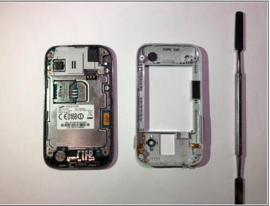
• Use the metal pry tool to separate the interior back panel from the interior hardware and screen.
