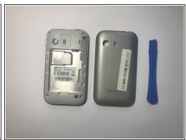
• Use the blue plastic opening tool to pry the back-panel off of the device.
