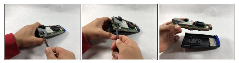
• Carefully pry the grey frame off the black plastic covering using the nylon spudger.
