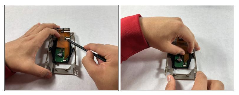
• Detach the remaining two orange flaps from the circuit board that is attached onto the grey frame.
