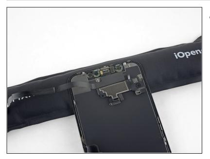
• Use a hairdryer, a heat gun, or a <u>heated iOpener</u> applied to the top front of the display for about a minute, in order to soften the adhesive securing the sensors.
