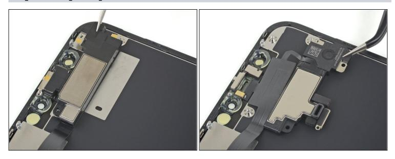
• Using tweezers, gently flip the speaker assembly over—down and away from the top edge of the display.
