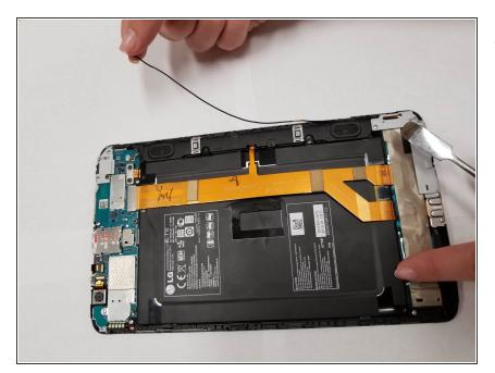
• Pull the cable back and out of the way of the speaker.
