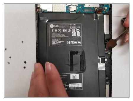
• Place spudger under the battery and run it around the edge to loosen it.
