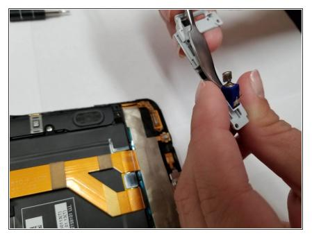
• Remove the vibrator from the underside of the white panel.
