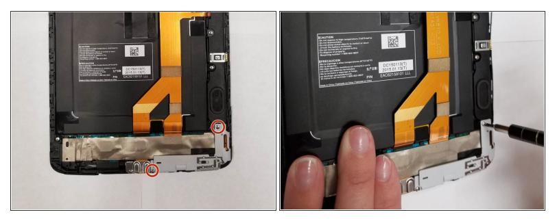
• Remove the two screws on the white panel on the bottom right side.
