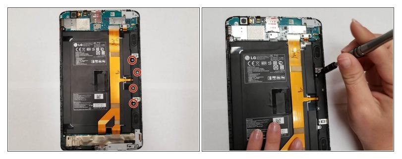
• Remove the 4 1.5 mm screws holding the speakers in place.
