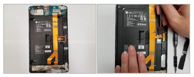
Insert metal spudger under the side of the gold strip and pull.
