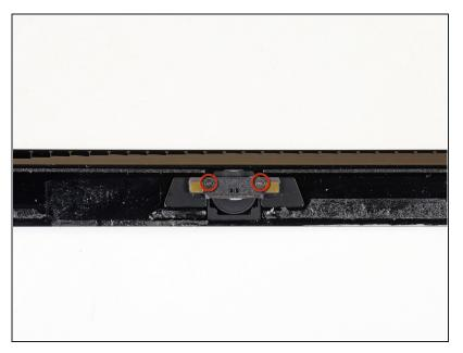
Remove the two 2.1 mm Phillips #00 screws securing the home button control board to the home button assembly.
