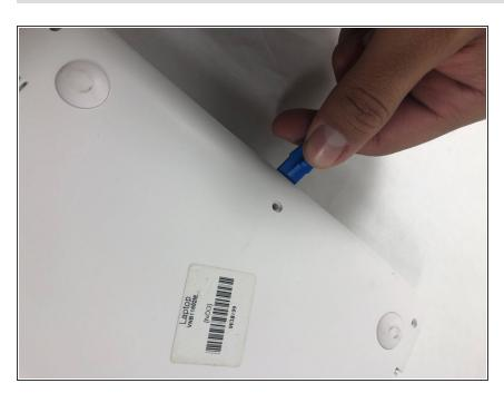
Use the iFixit plastic opening tool to put in between the lining of the back panel and begin to pry open the panel.
