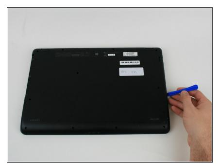
Run the opening tool along the bottom cover seam.
