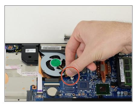
Unplug the clip (red black yellow wires) by pulling it in an upward direction.
