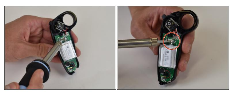
• <u>Desolder</u> the battery connections from the motherboard.
