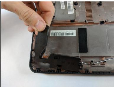
Use the plastic opening tool to release the speaker from its position.
