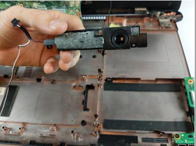
After the speaker is completely out, gently remove the wire that is attached to the speaker.
