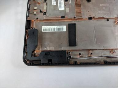
Speakers are located on the bottom left hand side of the device.
