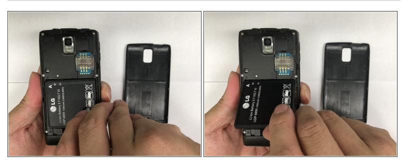
• Remove the battery by lifting from the bottom.
