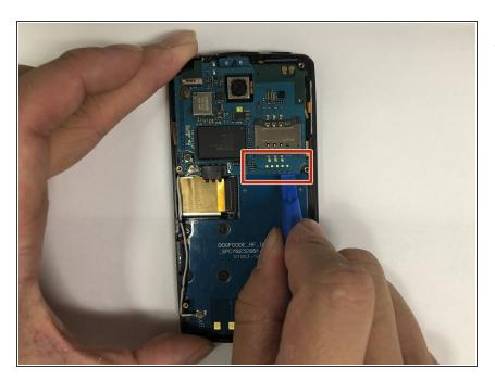
Pry off the connector using the iFixit opening tool to remove the communication board.
