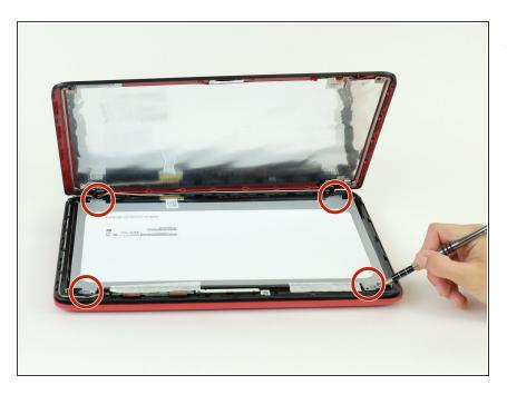
Use the Phillips #0 screwdriver to remove the four screws around the screen.
