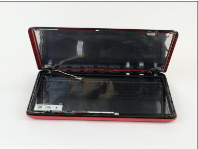
Unclip wire from the screen and lift screen to remove.
