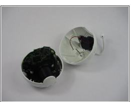
Take your tweezers and gently pull the white tip that is on the end of the white wire (the antenna) out from its plug in.
