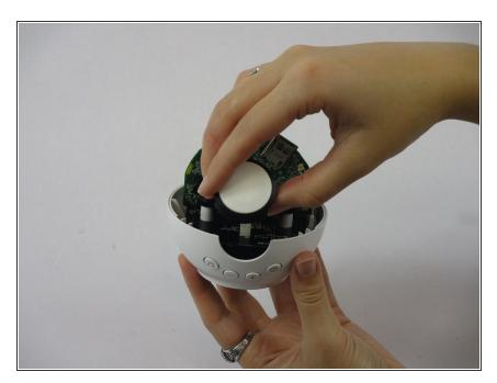
Gently lift the cylinder up from its placement in your Wi-Fi Baby Camera.
