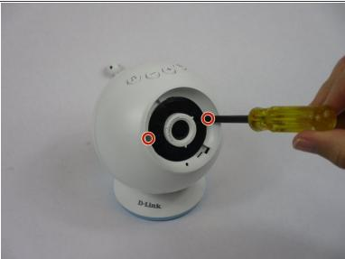
• Remove one Phillips #2 screw from each side of the camera lens.
