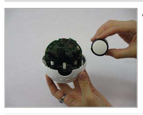
Remove the white cylinder completely to replace it.
