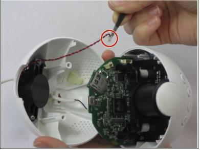
Take your tweezers and gently pull the white tip out from its plug that is connected to a red and black twisted wire.
