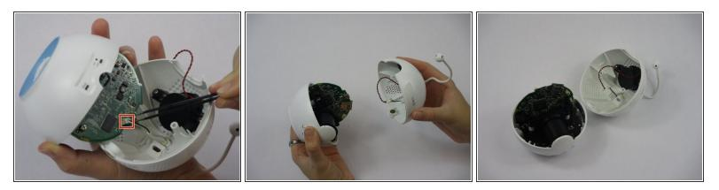
Take your tweezers and gently pull the white tip that is on the end of the white wire (the antenna) out from its plug in.
