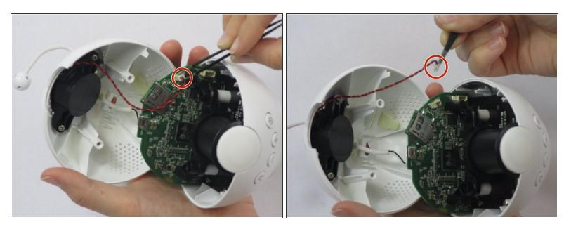
Take your tweezers and gently pull the white tip out from its plug that is connected to a red and black twisted wire.
