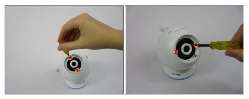
Remove one Phillips #2 screw from each side of the camera lens.
