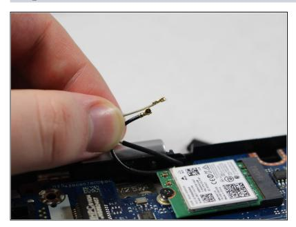
• Remove the wires attached to the WIFI card.
