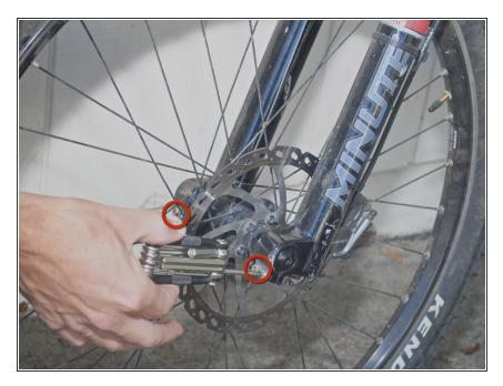
Using the 4mm Allen wrench, partially unscrew the 4 (22mm) hex screws on the front of the axle casing to allow the axle to slide freely.
