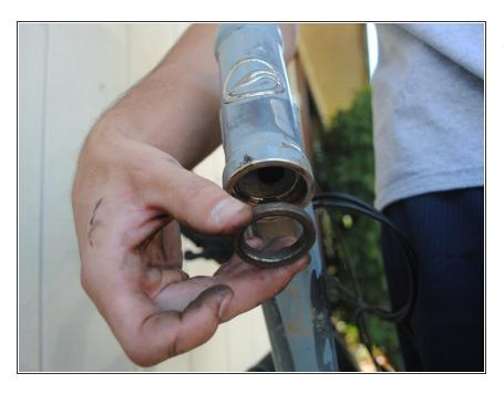
Using your fingers, pry the bearings from the top and bottom of the headset.
