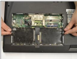
Gently pull on the tabs to lift the SD Hard Drives out of the computer.
