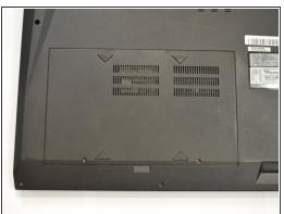
With the bottom of the computer facing up, remove the two 7.1 mm screws using a Phillips #00 screwdriver.
