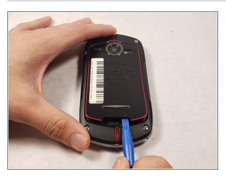
Using a plastic opening tool, gently lift open the back panel from bottom of the panel.
