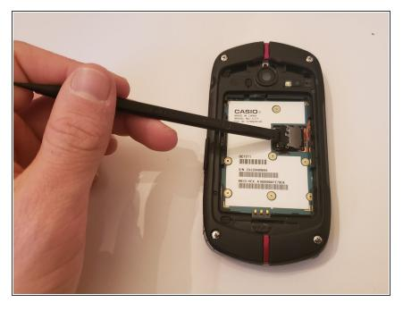
Using a spudger, gently open the metal tab up. Now, it is ready for you to insert the new SIM card.
